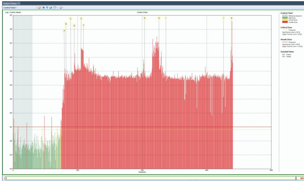
Figure 12. Fusion of damage indicators in a Hotelling T2 control chart, S101 bridge
