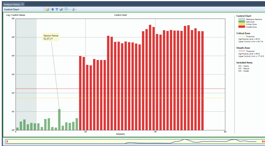
Figure 7. Fusion of damage indicators in a Hotelling T2 control chart, Z24 bridge
