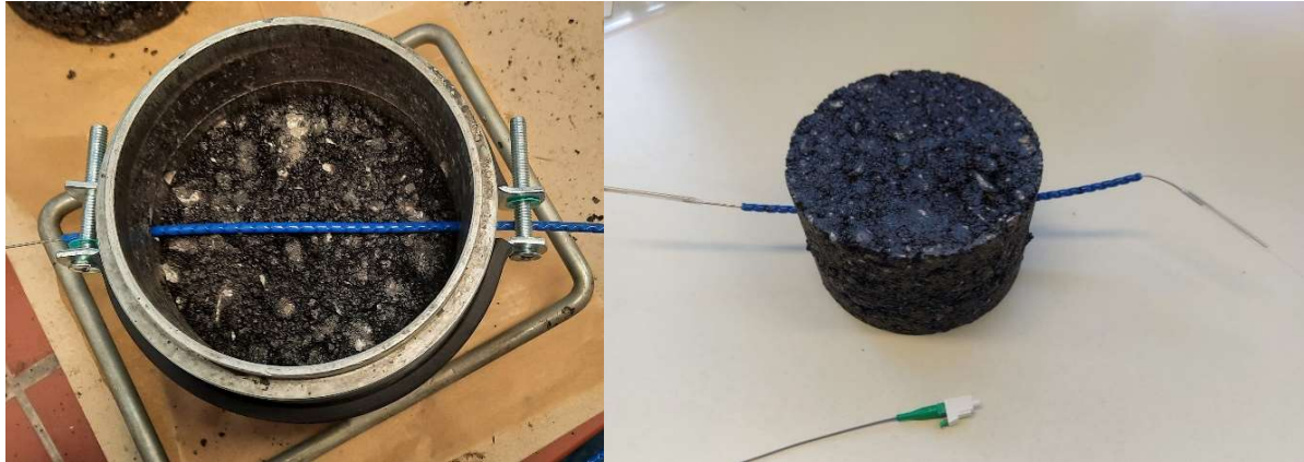
Figure 3. Lower half of the specimen with V9 cable (left) and full specimen with cable (right).
