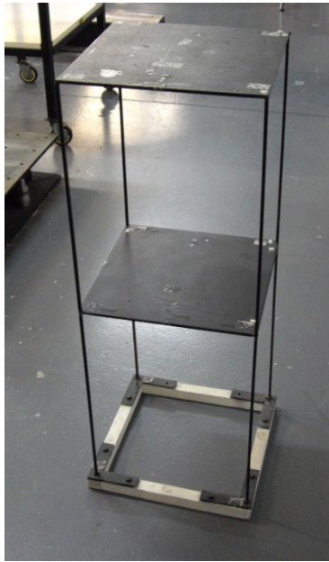
Figure 5. Two-floor steel frame structure.
