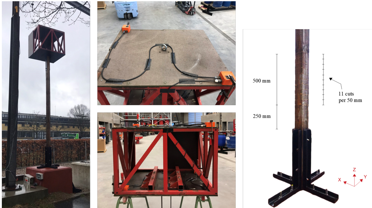
Figure 1: Left: Experimental model; Top middle: Two sensors are clamped on the upper plate of the topside; Bottom middle: Steel topside with the four sensors clamped on the different corners; Right: Damage cases on the wooden mast.
